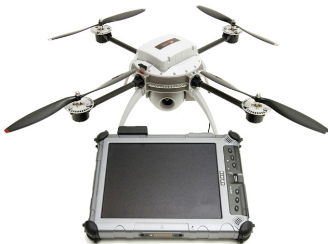
Figure 1.1: The Aeryon Scout is an unmanned micro aerial vehicle, used for tactical, over-the-hill aerial intelligence. The platform is controlled by a touchscreen interface and is able to fly pre-planned flight paths using GPS positioning.
