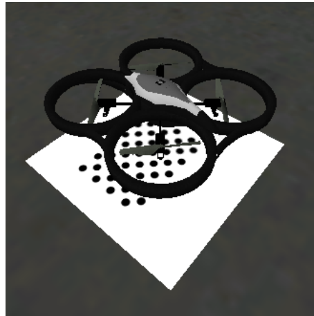
Figure 6.2: Calibration of a virtual camera inside the USARSim simulator.
