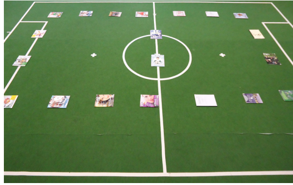
Figure 8.4: Photo of the texture-rich floor used for the first experiment. Magazine are spread out on the floor to provide sufficient texture. The dimensions of the 8-shape are approximately 5m \times 2.5m .
